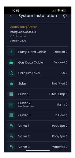
Enable data communication with Insrnrg Variable Speed Pump when green data cable connected between Chlorinator or Relay Hub controller and pump. When enabled, select the model of the variable speed pump and the RPM of each speed setting.
