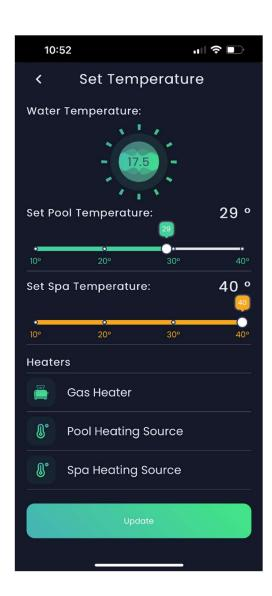
If more than one heater is installed and assigned to the Insnrg Controller, and you have a automated spa as part of your swimming pool, you can select which heater is used to heat the pool and which heater is used to heat the spa.
